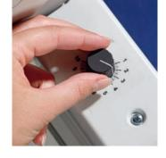
The conveyor speed is continuously adjustable and thus adapts without any problem to the letter length and the speed of your Frama Matrix franking system. After the last franking operation, use fast forward mode to stack the remaining letters in less than three seconds.
